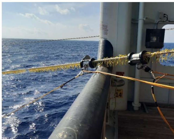
Figure 11. Slide collar over the lead-in (during deployment)
