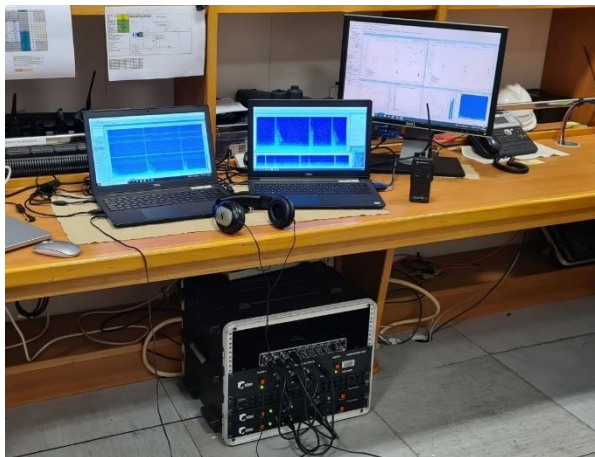
Figure 7 PAM monitoring station in the instrument room of the SW Cook (Credit: MFO/PAM Team)
