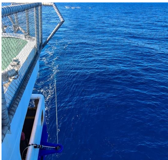
Figure 10 PAM hydrophone array cable deployment (Credit: MFO/PAM Team)
