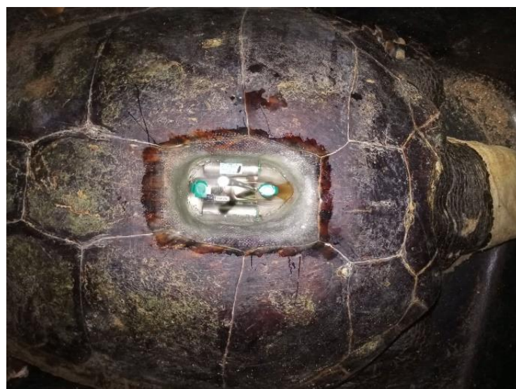
Figure 3-11. Detail of the transmitter in place on the turtle's carapace
