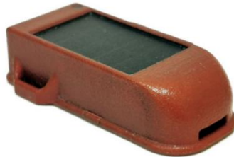
Figure 3-13. GPS-GSM device used for Scopoli's Shearwater telemetry
