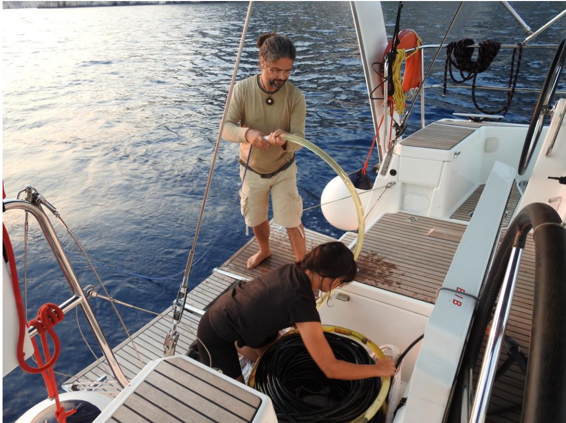
Figure 3-4. Part of the hydrophone array towed behind a sailing boat
