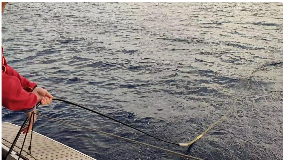
Figure 3-3. Part of the hydrophone array towed behind a sailing boat
