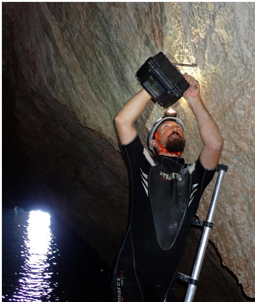
Figure 3-7. Installation of infrared camera systems in a monk seal shelter
