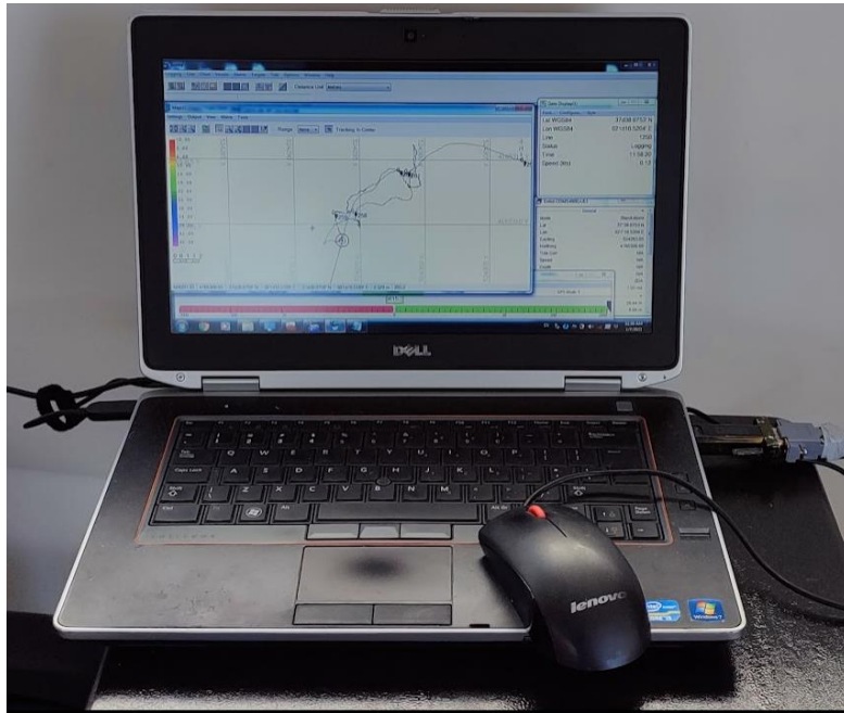
Fig. 2.1.2.4. Hypack 2014 navigation software on-board the research vessel.
