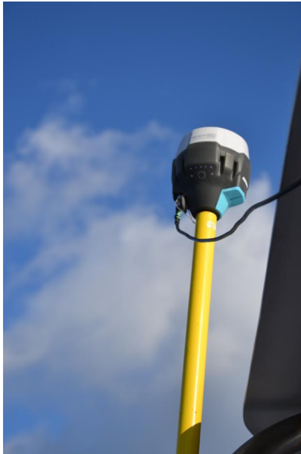
Fig. 2.1.2.3. The EMLID Reach GPS.
