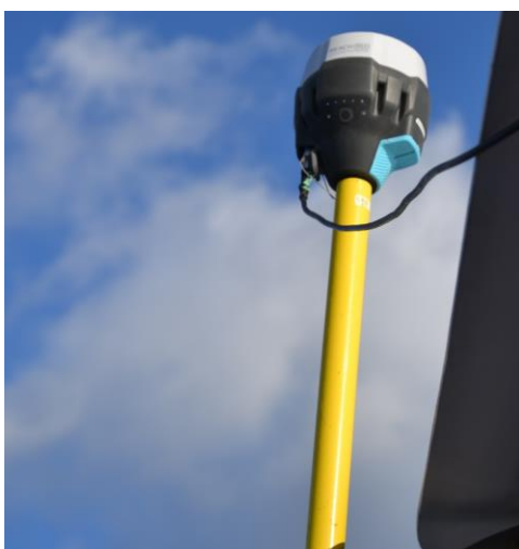
Fig. 2.1.2.3. The EMLID Reach GPS.
